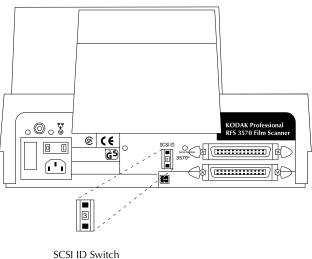
Each SCSI device connected to the same computer must have a different SCSI ID number. Your Macintosh Computer is number 7, and your internal hard disk is probably 0. If your computer has a CD-ROM drive, be certain to avoid its number also; it may be number 3 if it is an internal drive supplied by Apple Computer, Inc. Therefore avoid numbers 0, 3, and 7 since the Scanner must have a unique SCSI ID.
